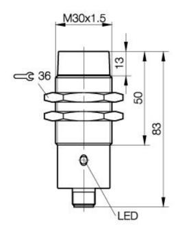
**Inductive Sensors** BES 516-549-S 4-H M30x1.5 x 83 normally-closed Sn=15mm unshielded
